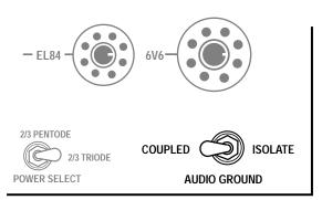
and two internal. The internal Grounds are the common zero voltage points for the power supply and audio circuitry. The external Ground is the safety connection of the metal chassis to your home's Ground Circuit.
